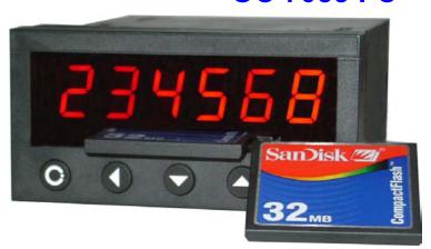
OC7053 FC is a 6 digit programmable Datalogger for connection to serial data ports RS232, RS422 and RS485.
